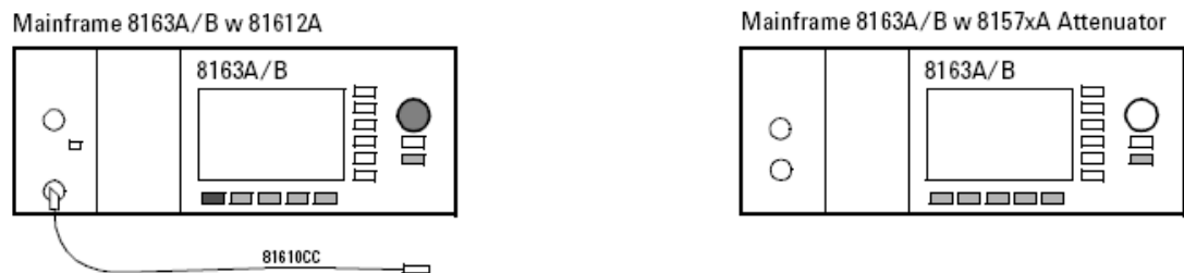
Figure 11 Return Loss Reference Setup for SM attenuators
